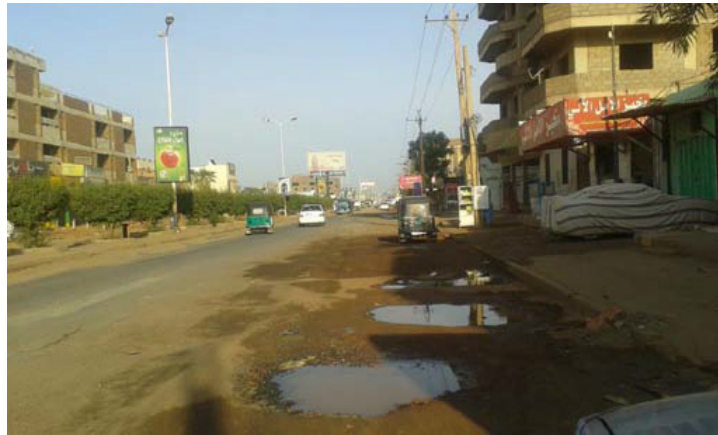
Fig. 5 Water Ponding on Potholes [5]
