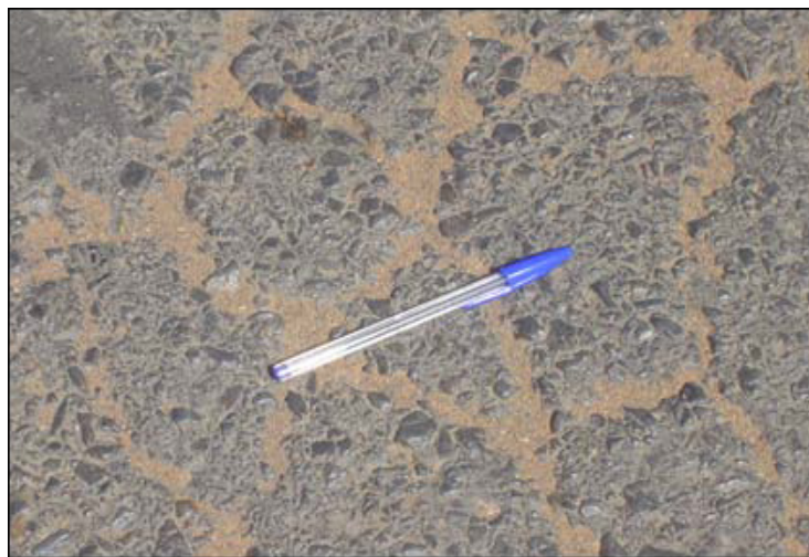
Fig. 3 Alligator cracking of high severe level [5]
